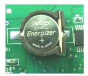
First Install battery for RTC , " + " mark on top
