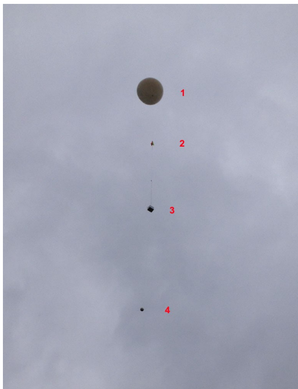
1. Balloon 2. parachute 3. Pi-HAB 4. Back-up Tracker
